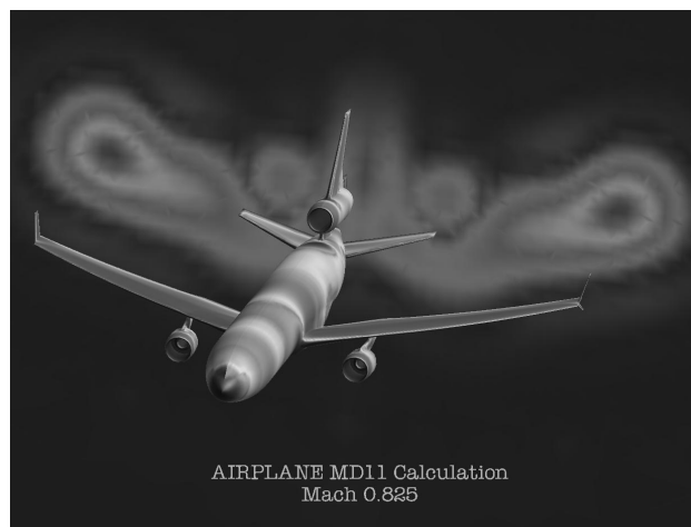
FIG. 12. Computed Pressure Field for a McDonnell Douglas MD11
